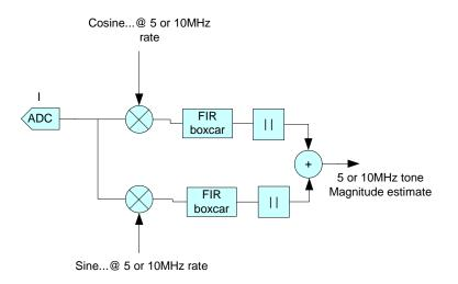
Figure 2. Quadrature conversion eliminates magnitude wandering due to phase variation.
