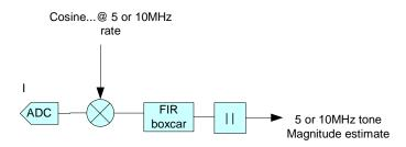
Figure 1 Digital down conversion and filtering to obtain an estimate of the magnitude of the detector 5 or 10MHz tone.
